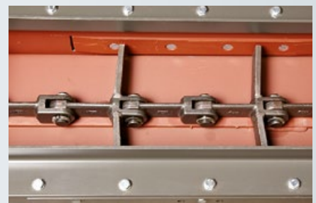
Drop-forged link chain for chain conveyor
