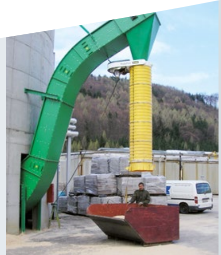
Loading facilities with chain conveyor and loading bellows
