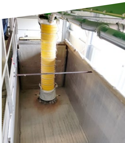
Low-dust loading of the sifted fine material
