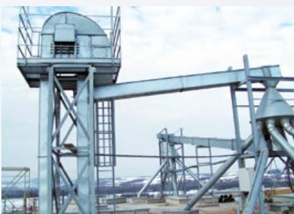
Product distributor comprising belt bucket elevator, chain conveyor and revolving tube distributor
