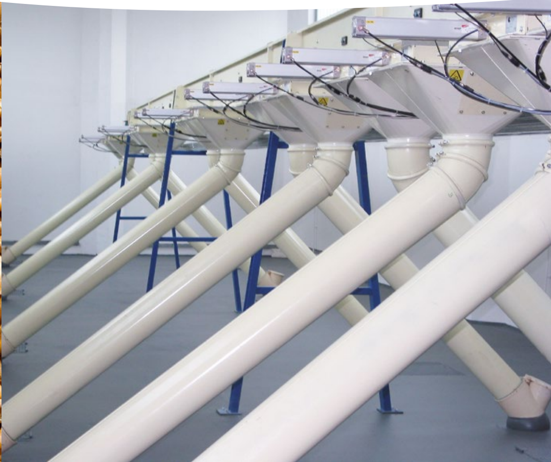
Silo bin feeding via chain conveyors and pneumatic gate slides
