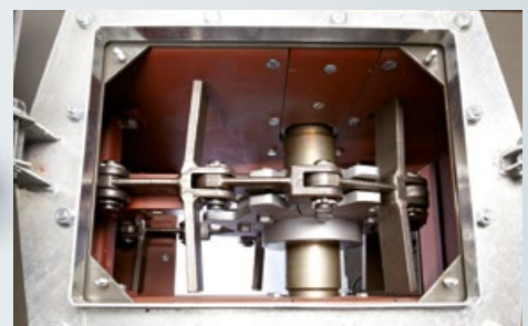
Drive system of a chain conveyor with drop-forged link chain
